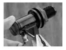
Where necessary bend the lever arm to adjust the water level. This can be done by removing the lever arm assembly by first straightening the tabs on the end of the pivot pin with a pair of pliers then slide it out.
