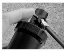
Insert the cam end of the lever assembly into the valve plunger recess. This may require rotation of the plunger to align it to the correct position. Align the cam hole with the valve housing and insert the pivot pin then flare the ends to secure.
