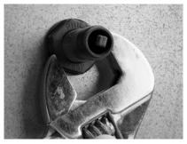
3. Screw the back nut onto the thread and tighten.
