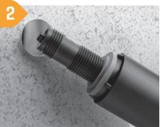
Screw into female thread by hand until firm.
