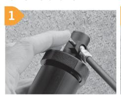
Apply PTFE tape or approved sealant to the inlet thread ensuring sufficient is applied to ensure a watertight seal.
