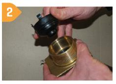
**Low Pressure Applications (LP)** - Remove the High Pressure insert to make the valve low pressure.
