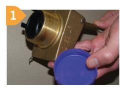
Remove protective cap and dispose. Note the high pressure [HP] insert in the valve body.
