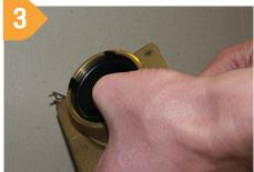
**High Pressure Applications (HP)** - Push insert into the valve body until lugs click into place. Valve is no suitable for high pressure.
