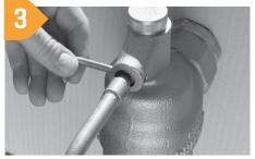
Remove the pivot pin from the body and fit the lever arm then ensure the pivot pin tabs are flared outward by using a small screwdriver.
