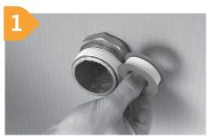
Apply PTFE tape or approved sealant to the inlet thread ensuring sufficient is applied to ensure a watertight seal.
