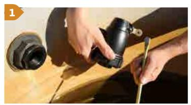
Unscrew bolt and remove lever from the float valve body.
