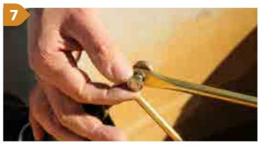
Then attach the upper lever which has ratchet slots for adjusting and locking the float at suitable level for your tank.
