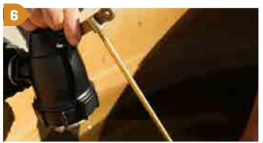
Attach the lower lever first by screwing the lever into the cam.
