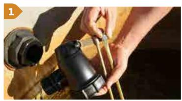
Remove both levers from the float valve body. Upper lever, remove fastening bolt.
