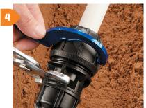
Tighten nut firmly with a wrench. Nut will not butt against the body flange when the pipe size is at the top end of the fitting tolerance.
