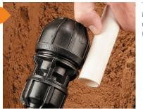
To ensure adequate insertion depth, witness mark the pipe to the back of the flange.
