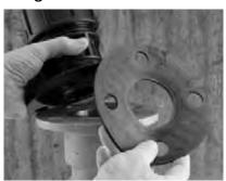
**I.** Ensure a gasket is used between the flange of the ratio valve and the flange to which it is to be fitted.
