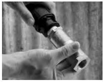
**2.** Screw into male thread by hand until firm.
