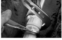
4. Nut tightening: Tighten nut firmly with a wrench. Nut will not butt against the body flange when the pipe size is at the top end of the fitting tolerance.
