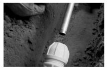
2. Ready to use position: The fitting is preassembled and ready to use, however always ensure the nut is backed off and 3 threads are showing. Pipes at the top end of the fitting tolerance may require 5 threads showing
