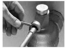
**6.** Remove the pivot pin from the body and fit the lever arm then ensure the pivot pin tabs are flared outward by using a small screwdriver.
