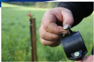
2. Insert the bolts into the saddle bottom and push firmly into the hex recess.
