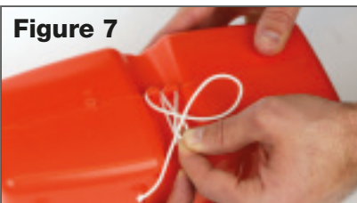
Loop the cord around the opposite lug and then pass through the loop
