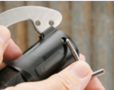
1. For overhead installation the lever needs to be relocated by unscrewing the pin from the body.
