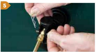
Where necessary bend the lever to adjust the water level. This can be done by removing the R-pin, sliding out the pivot pin and removing the lever.
