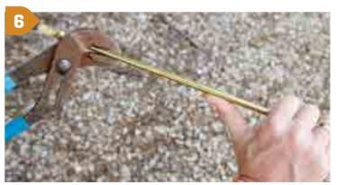
Using a pair of multi-grips or over a solid surface bend the lever to the necessary angle, then replace the lever.
