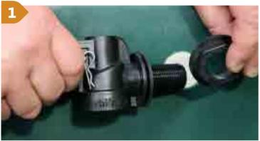
Remove back nut (rubber washer remains) and slide the thread through the appropriate sized hole.
