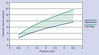
The above graph shows the performance of the nozzle in both washdown and wide jet full flow operation. The graph is based on testing carried out at RX Plastics.
